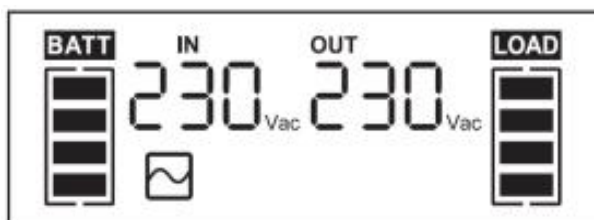
Fig. 9. Display in normal mode.
