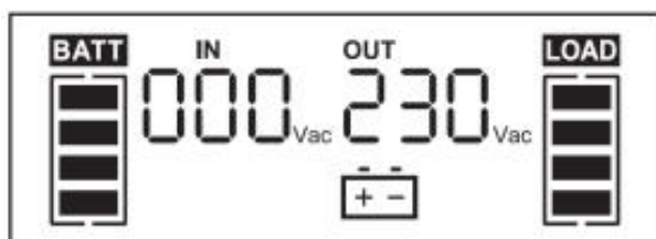
Fig. 11. Display in battery mode.
