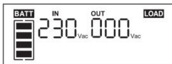
Fig. 12. Display in battery charger mode.
