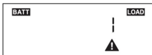
Fig. 13. Display in fault mode.
